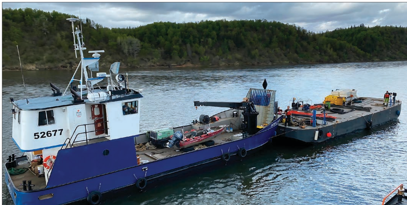
The tug Jackie M pushes a small fuel barge. These vessels are small, shallow-draft assets serving the upper villages of the Nushagak River in Alaska. The twists and turns of the upper river require small equipment. Photo courtesy of Vitus Marine
