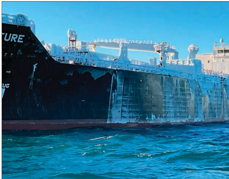
Rough seas, freezing temperatures, and ice accumulation on vessels are daily challenges of working in some of Alaska’s most remote locations. Severe ice accumulation can cause dangerous stability issues. Coast Guard photo by CWO4 Shawn Erwin
