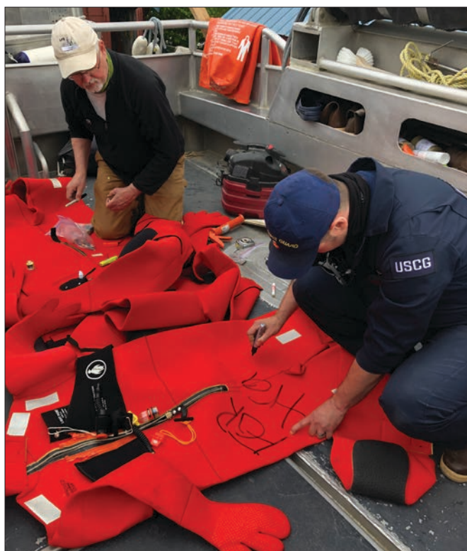
During safety equipment checks on board fishing vessels, inspectors examine immersion suits for failures, flaws, or damage. While conducting these examinations, a sector reservist found a manufacturing defect that culminated in the company issuing a recall of the suit. Coast Guard photo by Petty Officer 2nd Class Holly Bernosky
